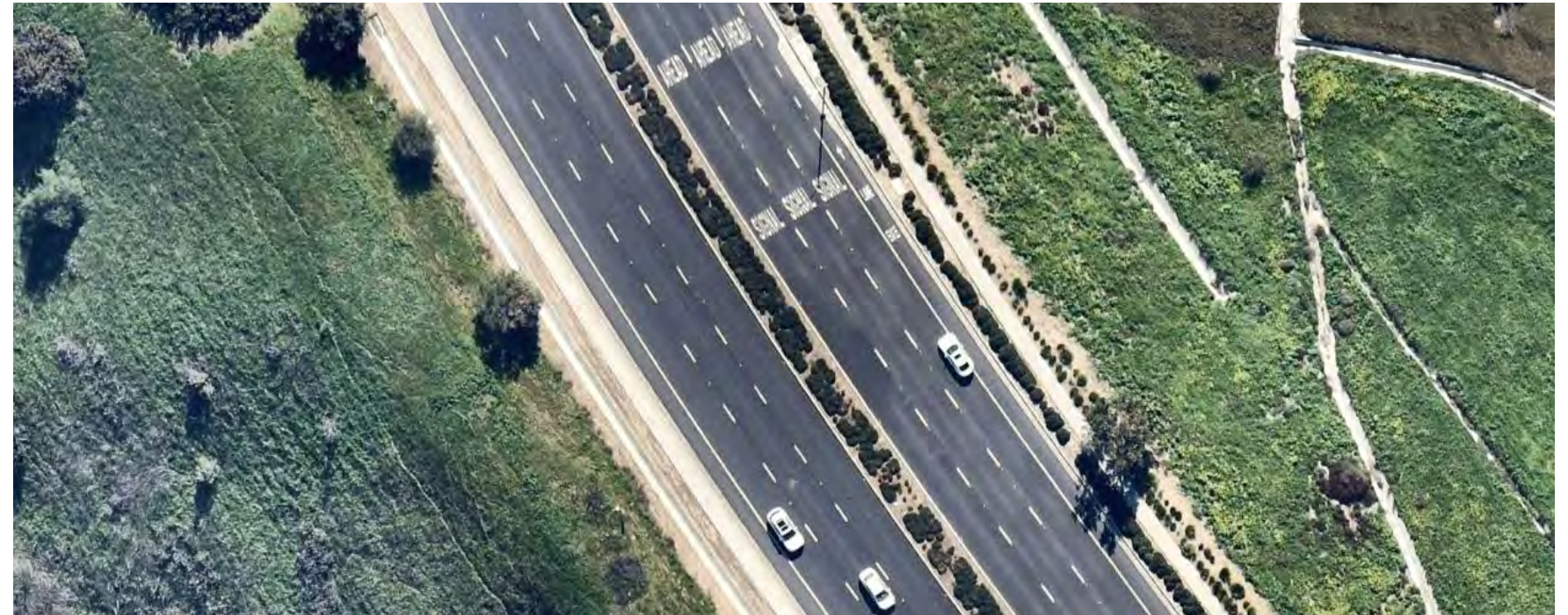
Antonio Parkway has three travel lanes in either direction, and existing Class II bike lanes
