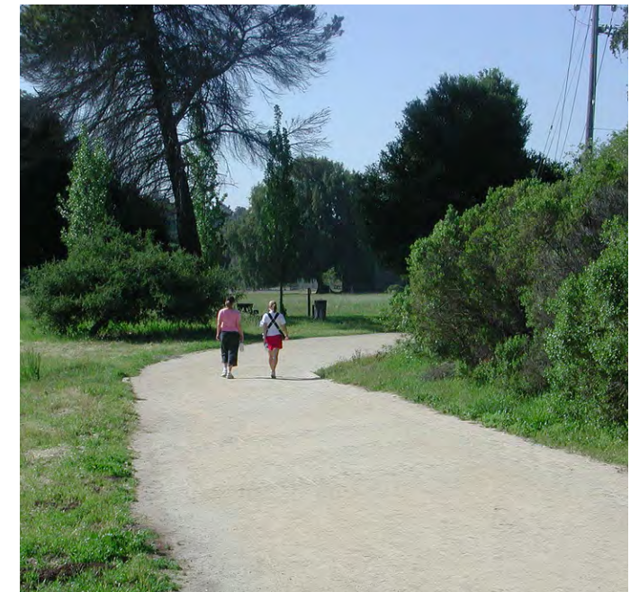
Decomposed Granite (DG) Pathways: provide a natural but stable pathway surface.
