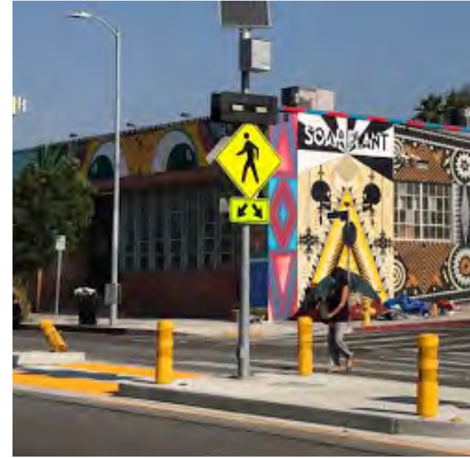
Pedestrian Refuge Islands: allow pedestrians to stop before finishing crossing a road.
