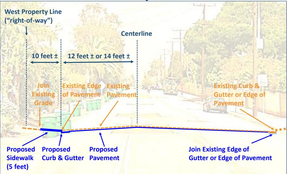
North of Rainier Dr.: Proposed west-side curb to existing east-side edge of pavement: ± 24 feet. Proposed west-side curb to centerline: ± 12 feet.
